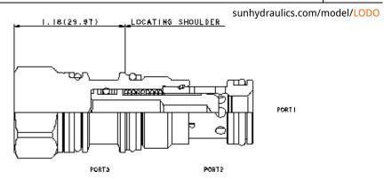
These unbalanced, pilot-to-close logic valves are 2-way switching elements that are spring biased open. Pressure at either work port 1 or 2 will tend to keep the valve open while pressure at port 3 will tend to close it. The force generated at port 3 must be greater than the sum of the forces acting at port 1 and port 2 plus the spring force for the valve to close. NOTE: The pilot area (port 3) is 1.8 times the area at port 1 and 2.25 times the area at port 2.
