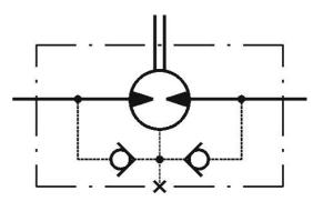
The shaft seal pressure equals the pressure in the drain line
