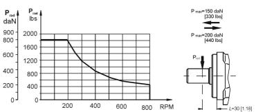
Radial Shaft Load Prad for C,CO Shaft Extensions by L=30mm[1.81in]
