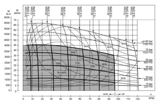
The function diagrams data is for average performance of randomly selected motors at back pressure 5÷10 bar [72.5÷145 PSI] and oil with viscosity of 32 mm²/s [150 SUS] at 50°C [122°F].
