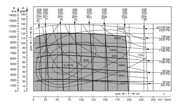
The function diagrams data is for average performance of randomly selected motors at back pressure 5÷10 bar [72.5÷145 PSI] and oil with viscosity of 32 mm²/s [150 SUS] at 50°C [122°F].
