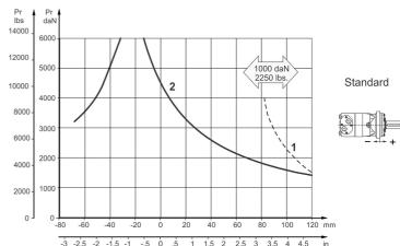
Curve "1" shows critical radial shaft load. The output shaft runs in tapered bearings that permithigh axial and radial forces. The permissible radial loadon the shaft is shown (curve 2) for an axial load of 0 Nas function of the distance from the mounting flange to the point of load application. The curve 2 apply to a B10 bearing life of 2000 hours at 100 RPM.
