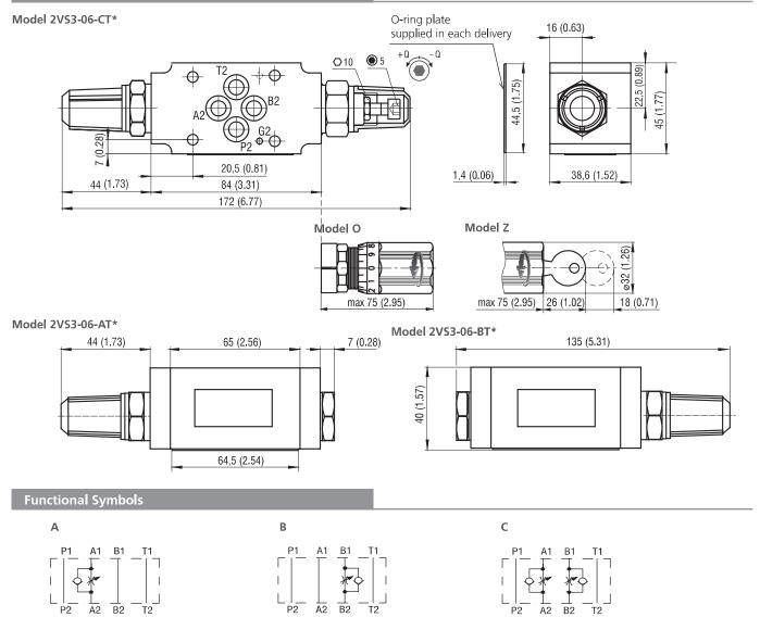
**Notice:** The orientation of the symbol on the name plate corresponds with the valve function.
