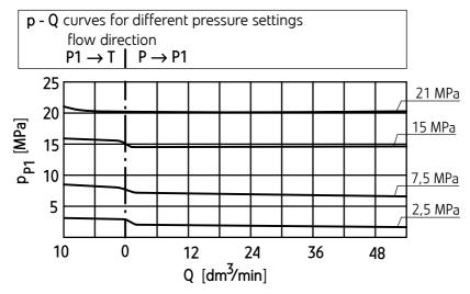
Characteristic curves of minimum pressure drop in relation to flow rate in the direction of flow P - P1
